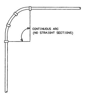
For plastic conduit, use 15-foot (4.6 m) radius bends (7 or 30 degrees, as required). Rigid bends are described on Pages 8-24 and 8-25.
