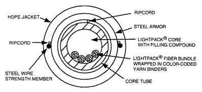
The *Lightpack* cable bundle identification is made possible by the application of 2 spirally wrapped color-coded yarn binders around each bundle. The following colors are used to identify bundles.
