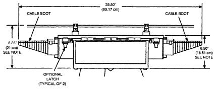
NOTE: CABLE TERMINALS EQUIPPED WITH 25 PAIR PROTECTED BLOCKS HAVE AN EXTENDED TERMINAL REGION WHICH ADDS 1.75" (4.44 cm) TO THESE DIMENSIONS
