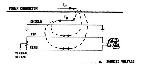
If the opposing voltages were equal, shielding would be perfect. In practice, shielding is most effective when the total resistance of the shield circuit (shield resistance and resistance to ground) is as small as possible. It is important to ensure and maintain cable-sheath continuity and low resistance to ground.
