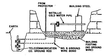
Acceptable Protector Grounding Connections when Power Service is not Grounded, Power Service Grounds not Accessible, or there is no Power Service at the Premises
