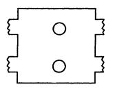
For the same depth and type of racking, a center rack manhole is twice as wide as a basic manhole and can accommodate twice as many main cables.
