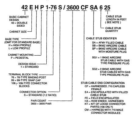
NOTE: STUB LENGTHS ARE AVAILABLE IN 20- TO 100-FOOT LENGTHS IN 10-FOOT INCREMENTS TO BE SPECIFIED ON ORDER AS E/W XX FT. STUB.
