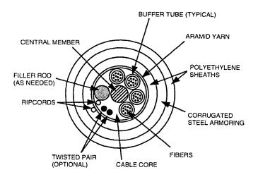
The cable core consists of a number of buffer tubes, each containing from 1 to 12 fibers, surrounding the central member. The central member can be a dielectric epoxied glass rod or a steel rod with polyethylene buildup. High density polyethylene filler rods are installed as required to maintain the integrity of the cable core. A filling compound is applied to prevent water penetration and dual binder threads are used to secure the core.
