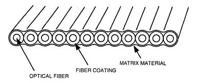
Fiber counts are available from 12 to 216 fibers for singlemode and 12 to 144 fibers for multimode (in increments of 12 fibers). Each fiber position is guaranteed. The ribbon stack is housed in an extruded plastic tube. The plastic tube's outer diameter is nominally 0.31 inch (7.9 mm) for fiber counts up to 96 and 0.41 inch (10.4 mm) for fiber counts from 108 to 216. Up to 18 ribbons can be contained in the core tube.
