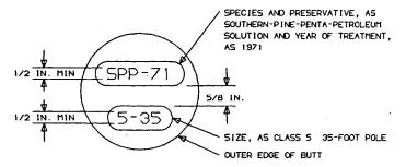
NOTE THE BUTT MARKING SHOULD BE LOCATED WITH RESPECT TO OUTER EDGE OF BUTT, APPROXIMATELY AS SHOWN
