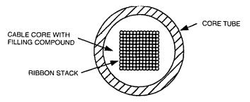
Each ribbon, in an *AccuRibbon* cable, has identifying marks consisting of a number (1-18) and a 2-letter color abbreviation (for example BL=blue) printed along its length every 6 inches (150 mm). The markings are printed directly on the ribbon structure and may be used for mid-span or end-entry identification.
