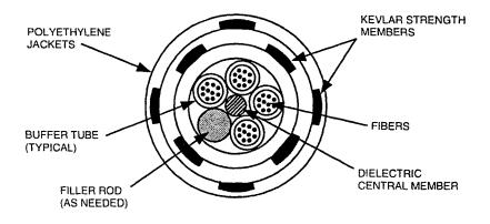
The physical characteristics of *PowerGuide* fiber optic cables are showr below:
