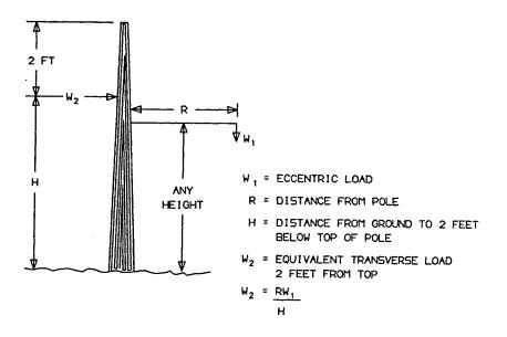
If the attachment is a conductor subject to ice coating, see AT&T 919-370-200 for the method of computing weight.
