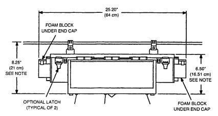
NOTE: CABLE TERMINALS EQUIPPED WITH 25 PAIR PROTECTED BLOCKS HAVE AN EXTENDED TERMINAL REGION WHICH ADDS 1.75" (4.44 cm) TO THESE DIMENSIONS
