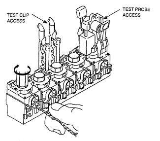
K-Series IDC Block With 22-Gauge (0.6 mm) or 24 Gauge (0.5 mm) Wire Inserted
