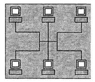
In a star topology, all of the nodes or workstations are connected with UTP or fiber optic cable to a centrally located common controller or concentrator. The central control point permits centralized network administration, management, and troubleshooting. StarLAN is an example of a star topology, as is IEEE 802.3
