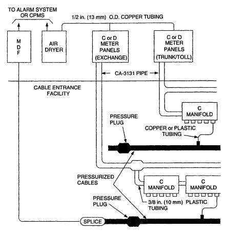
The outside plant portions of typical exchange and trunk/toll pressure systems are shown below. For details not shown here, see AT&T 637-225-201.
