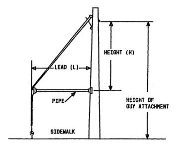
The strand size required for fabricating a sidewalk anchor guy must be larger than that required for an anchor guy of the usual type having the same lead/height ratio.
