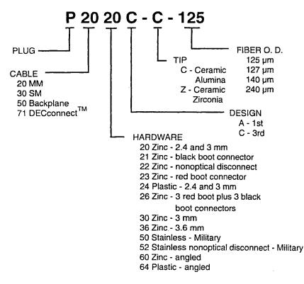
The coding scheme for the ST connectors is shown below:
