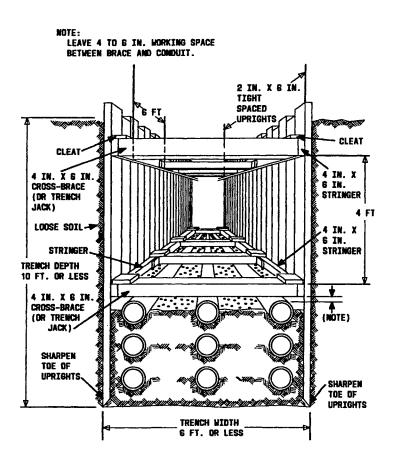
Trenches less than 5 feet (1524 mm) deep should be shored if they constitute a hazardous work location. Someone shall be stationed on the surface to keep the persons in the excavation in sight at all times.
