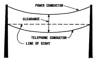
Note: For spans greater than 150 feet (45.7 m), the sag of opensupply conductors shall not dip below the line-of-sight between the telephone-conductor attachment-points at 60°F (15.5°C) with no wind displacement.
