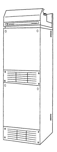
AUTOPLEX System 1000 — Series II Cell Site Cabinet (Radio Channel Frame/Linear Amplifier Frame [RCF/LAF])
