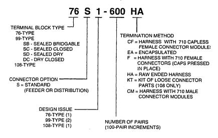
NOTE: STUB LENGTHS ARE AVAILABLE IN 20- TO 100-FOOT LENGTHS IN 10-FOOT INCREMENTS TO BE SPECIFIED ON ORDER AS E/W XX FT. STUB. ALL TERMINAL BLOCK WIRING, HARNESSING, AND CABLE IS 24 AWG (0.5 MM).
