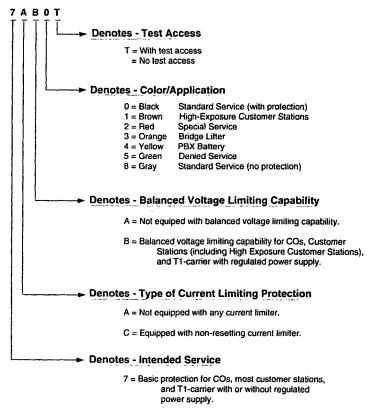
Note: The end of the housing handle is typically stamped with symbols to further identify type/application information.
