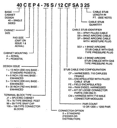
NOTE: STUB LENGTHS ARE AVAILABLE IN 20- TO 100-FOOT LENGTHS IN 10-FOOT INCREMENTS TO BE SPECIFIED ON ORDER AS E/W XX FT. STUB.
