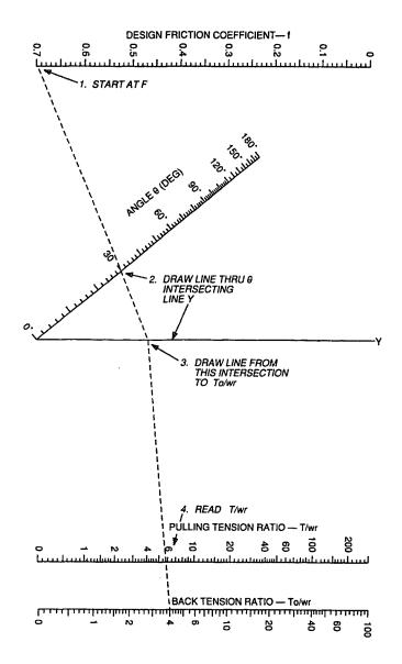
To find the pulling tension for a conduit section containing both straight and curved segments, calculate the tension segment by segment, starting at the feed (or reel) end.  $T_0$  is the tail load on the cable entering the duct. Use the calculated value of T found for the first segment by applying it as  $T_0$  for the second segment, and so on, until the pulling tension on the cable at the winch is obtained. A pulling tension problem is illustrated below.
