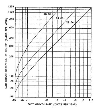
Add the duct growth rates for all gauges from the chart shown on Page 8-3; then, add the growth rates for trunk, toll, and other services. On the following chart, find the number of ducts for growth from the curves, using local "A" and "B" costs. ("A" cost is the getting started cost per trench foot and includes such items as permits and engineering. "B" cost is the cost per duct foot and includes such items as material and labor.)
