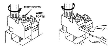
**Drop Wire Insertion for J-Series IDC Block**
