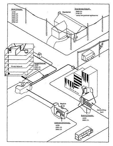
Below is a drawing showing typical applications of the specific AT&T closures.
